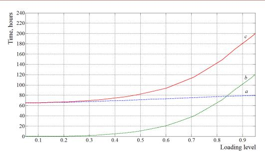
Picture 1. The dependence of the mean vessels cargo handling processing time (a), the mean waiting time in the roads (b) and the mean overall waiting time (c) from the loading level of the terminal
