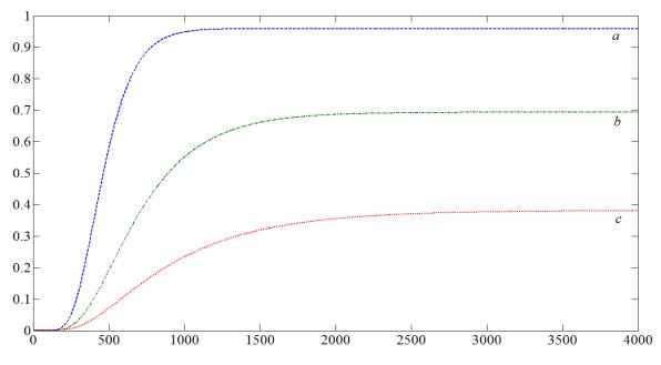
Picture 3. The change in the probability that at least one of the berths will be available if the loading level of the terminal (a) – equals 0,27, (b) – equals 0,6 or (c) – equals 0,82, and the road is overflowed at the beginning of the period.
